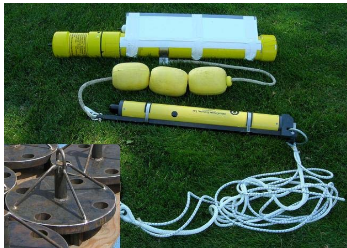
Figure 2. Autonomous acoustic telemetry receiver (top), acoustic release (middle), and anchor (bottom left) rigged as deployed in the Columbia River estuary.
