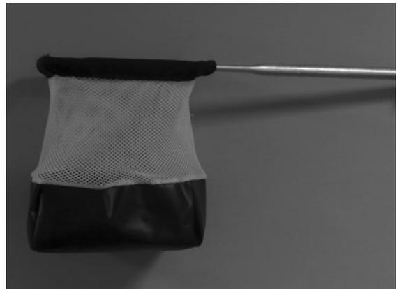
**Fig. 1** Sanctuary nets, used in fisheries research, are lined along the bottom with vinyl to retain water so fish are not air exposed and abrasion with net is minimized
